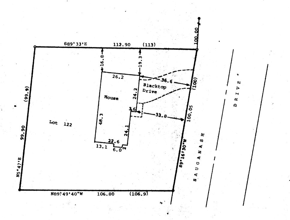
Scale - 1" = 20' o = 3/4 Dia. Iron Pipe Found • = Concrete Monument Found (000.0) = Recorded Distance Bearings are referenced to the Westerly line of Lot 122, recorded bearing of N5°47'E.
